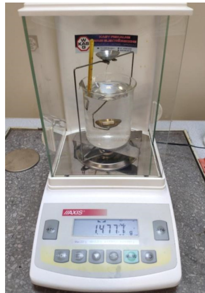
Figure 4. Density measurement system.
