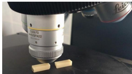
Figure 6. Geometric structure of the surface measurement of the sample surface near the fracture.
