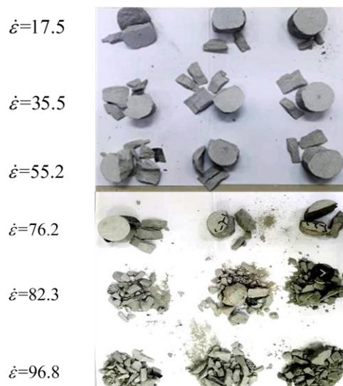
**Figure 9.** The failure modes of medium sandstone specimens from conventional dynamic uniaxial compression experiments.
