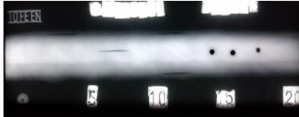
**Figure 25.** Radiogram of welded plate 3: 0–20 distribution.
