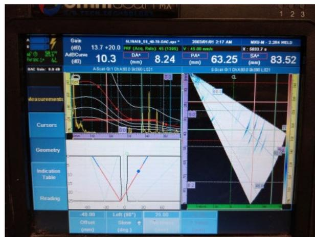
Figure 7. Welded plate—1: continuous signal 1.
