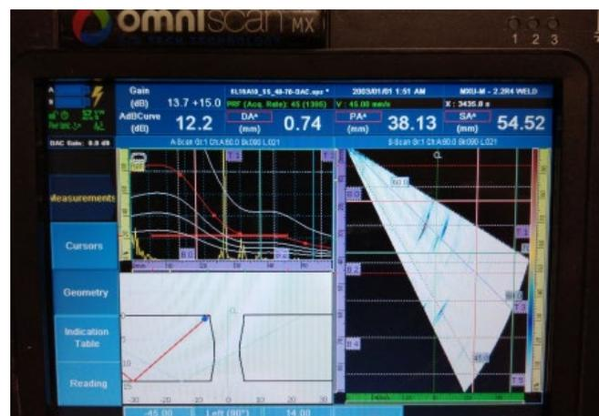
Figure 13. Welded plate—2: continuous signal 2.
