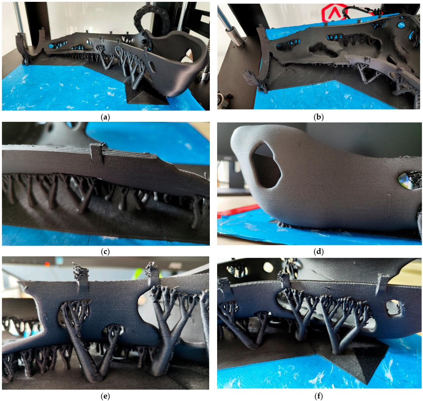
**Figure 15.** Fabrication of the greave using the outer shell as an example: (a) front view; (b) top view; (c) snap hook; (d) bottom view; (e) support structure; (f) isometric view.
