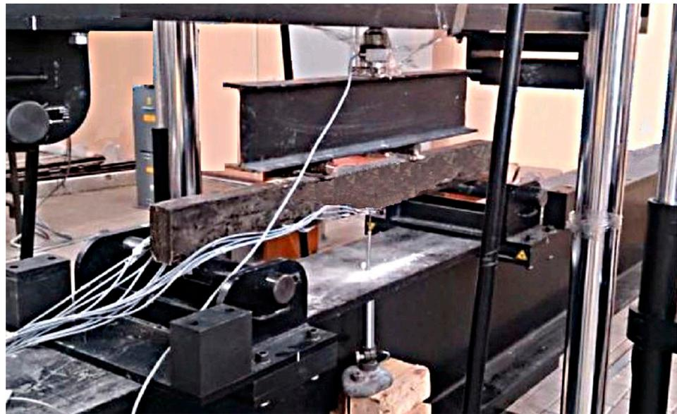
**Figure 2.** General view of the bending test of rubber concrete beams.
