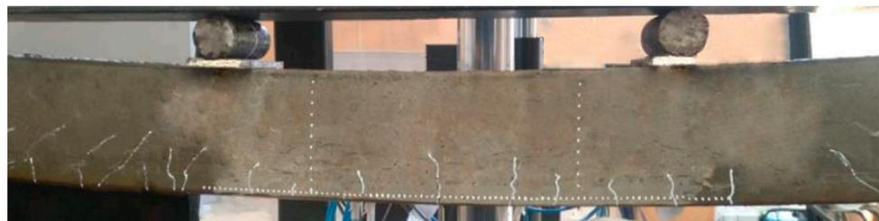
Figure 11. Fracture along the compression zone of the CPS beam.
