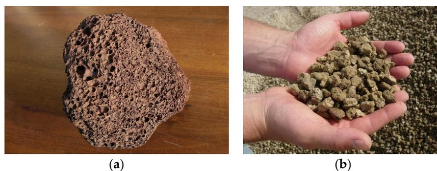
**Figure 2.** Lapillus (a) and zeolitic tuff (b) [16].
