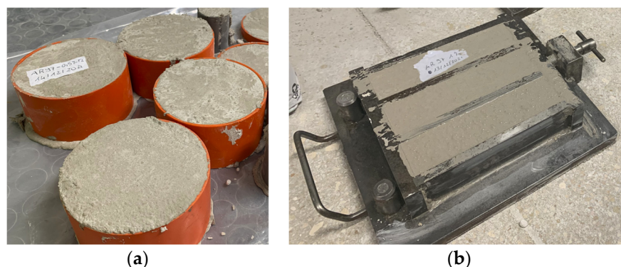
Figure 2. Molding of samples for non-destructive thermal conductivity tests (a); molding of samples for compression tests (b).
