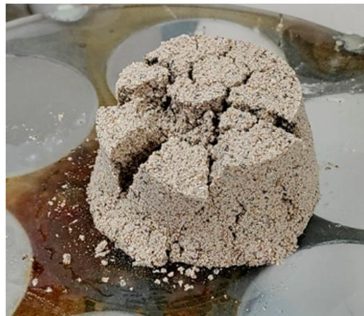
**Figure 6.** Appearance of the Labo CSA cement mortar on the shaker table.
