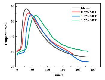
Figure 3. Internal temperature of concrete specimen.
