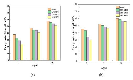
**Figure 2.** Compressive strength of concrete specimens at different ages. (a) is the compressive strength of concrete specimen under normal temperature curing; (b) is the compressive strength of concrete specimen under variable-temperature curing.
