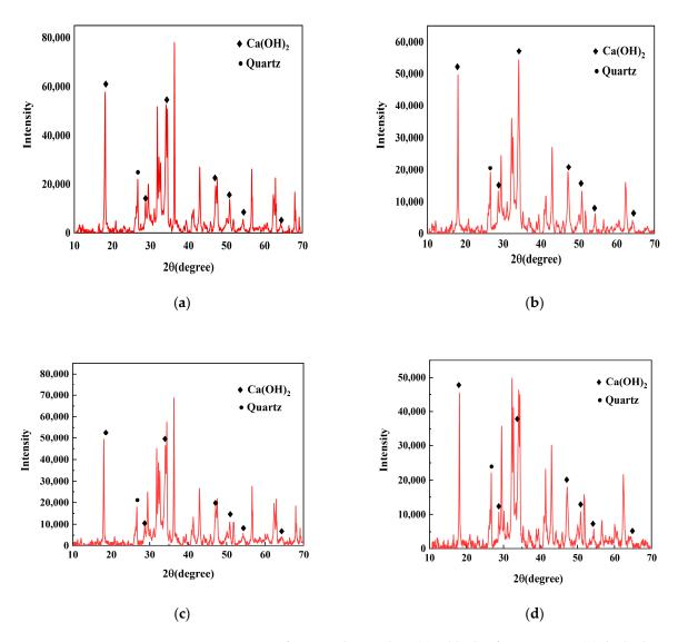
**Figure 5.** XRD pattern of cement slurry, where (a) is blank reference group; (b) the hydration temperature rise inhibitor group containing 0.5%SBT; (c) is the dosage of 1.0%SBT hydration temperature rise inhibitor group; (d) is the dosage of 1.5%SBT hydration temperature rise inhibitor group.
