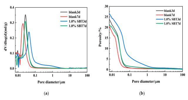
**Figure 8.** 3 d and 7 d mercury injection maps of blank cement paste group and 1.0%SBT. (a) is the aperture distribution diagram of each specimen; (b) is the cumulative aperture distribution diagram of each specimen.
