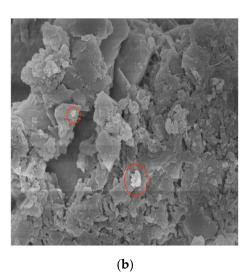
**Figure 9.** SEM image of 3 d concrete specimen. (a) SEM diagram of concrete specimen without water-added temperature rise inhibitor 3 d; (b) SEM diagram of concrete specimen doped with 1.0%SBT hydration temperature rise inhibitor.
