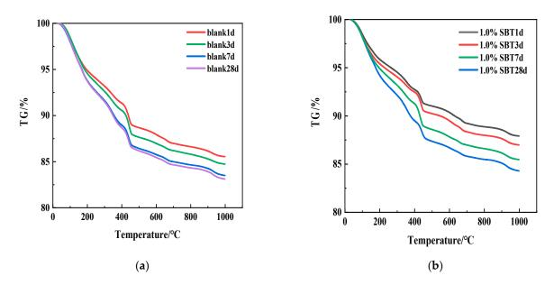
**Figure 6.** TG diagrams of cement slurry at 1 d, 3 d, 7 d and 28 d. (a) The TG curves of the blank group at 4 instars; (b) is the TG curve of 4 instars of hydration temperature rise inhibitor containing 1.0%SBT.
