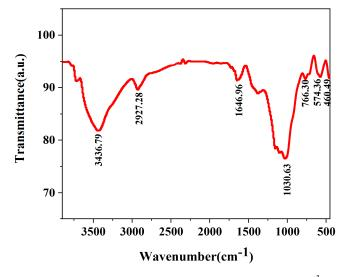
**Figure 1.** FTIR spectra of SBT with a resolution of  $0.4 \text{ cm}^{-1}$ .
