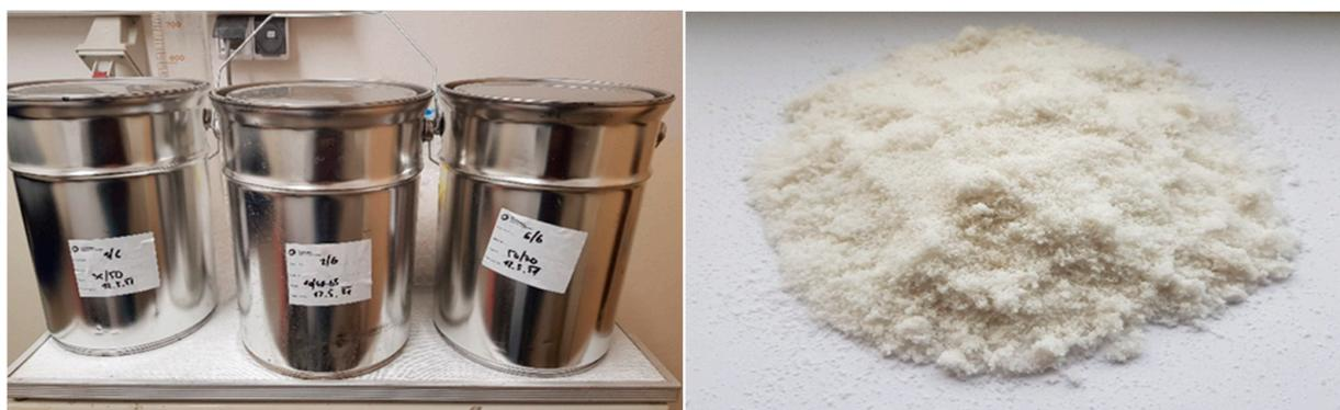
**Figure 1.** Materials for the first experiment of the interaction of straight run bitumen CA 35/50; 50/70 (left) and fast-reacting SBS polymer (right).
