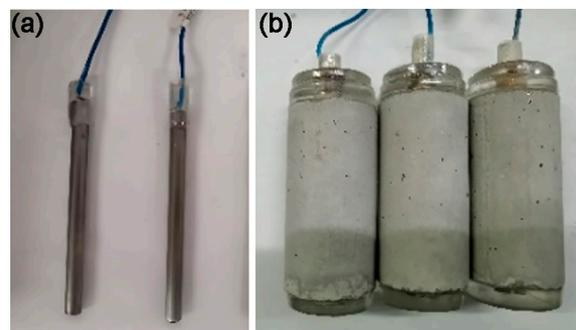
**Figure 1.** (a) the reinforcing bar welded with copper wire; (b) the LDHs incorporated mortar specimens with embedded reinforcing bar.
