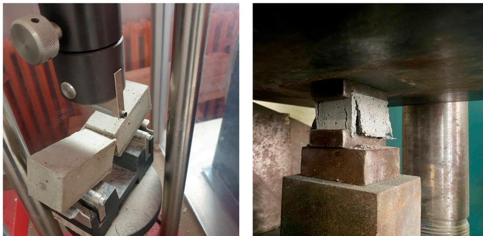
**Figure 4.** Determination of tensile and compression strength of hardened plastering mortars.
