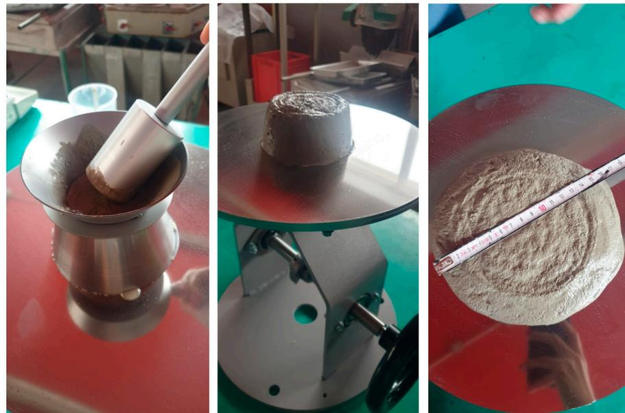
**Figure 2.** Fresh mixture testing to assess the consistency using the 16–17.0 cm diameter of the spread.
