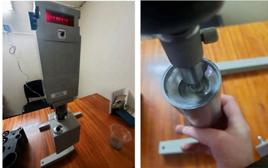
**Figure 3.** The mixed specimens during the test in the rotational rheometer RPE-1M.
