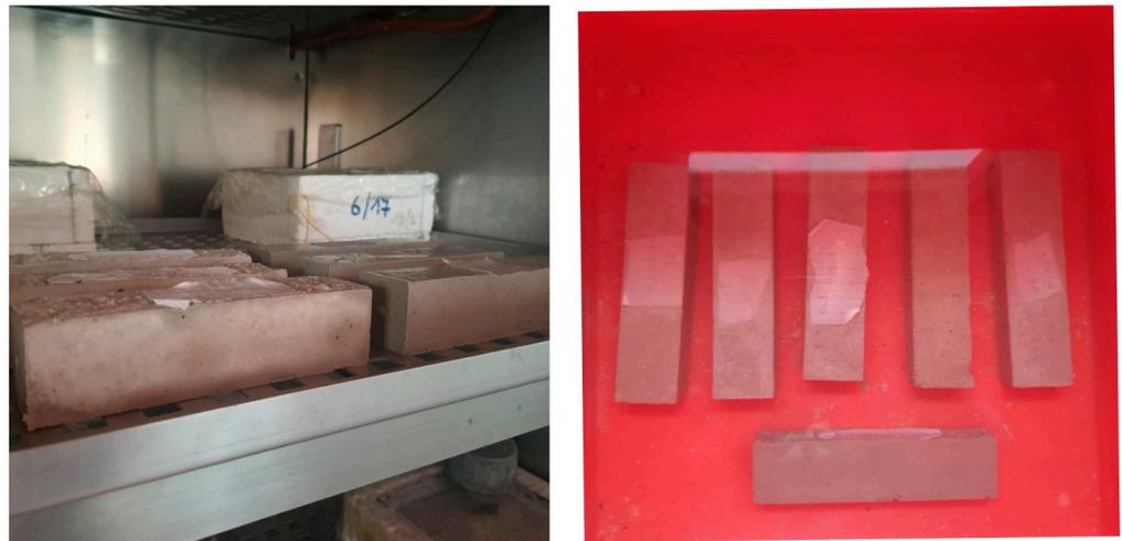
**Figure 5.** Determination of frost resistance. Specimens in a freeze chamber and in water for thawing.
