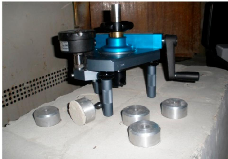
**Figure 6.** The specimens under adhesion strength tests using DYNA Z16 pull-off tester.
