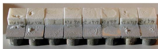
**Figure 3.** (a) Tensile bond strength of sprayed PUR foams after cryoshock test vs. NCO/OH ratio. (b) Sprayed PUR samples after cryoshock and tensile bond strength test.
