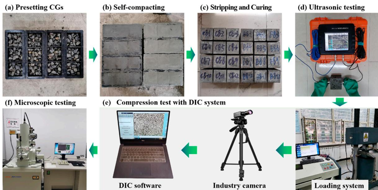
**Figure 2.** The preparation process and test methods on SCFB samples.
