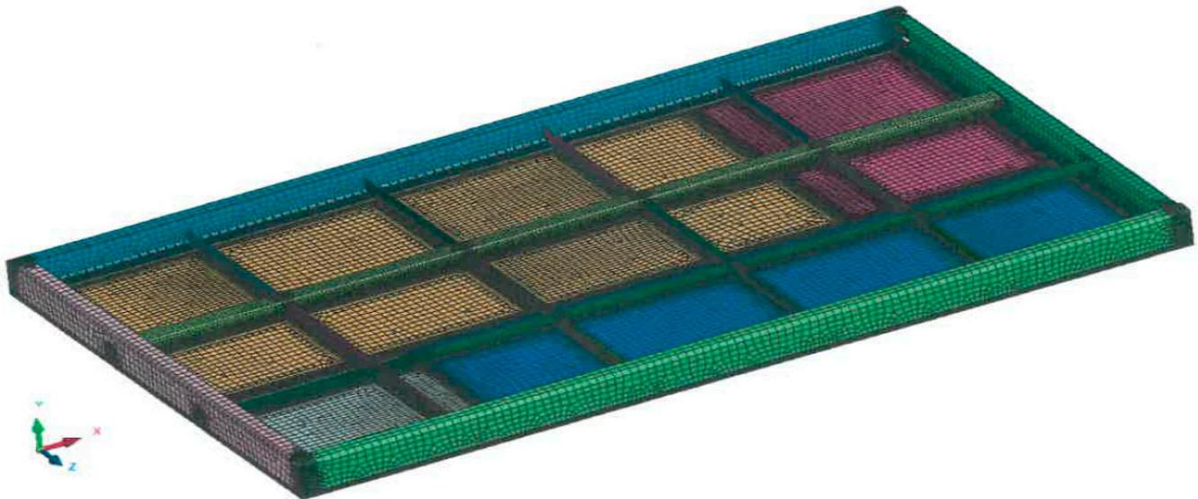
**Figure 2.** CAD and FEM model of the industrial furnace wall panel.
