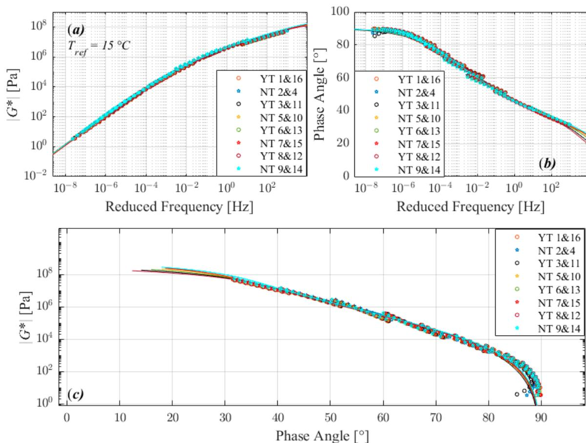
**Figure 3.** Comparison of master curves of complex shear modulus (a), phase angle (b), and black diagram (c) for 50/70.
