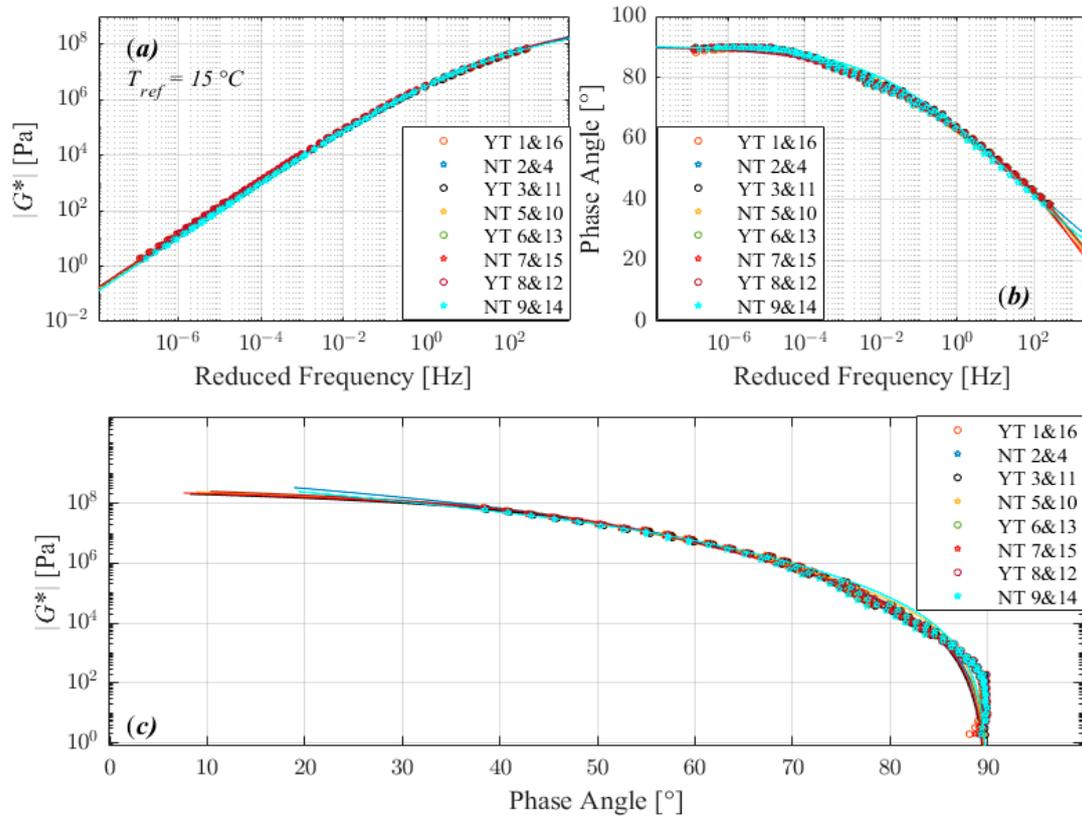
Figure 4. Comparison of master curves of complex shear modulus (a), phase angle (b), and black diagram (c) for 70/100.
