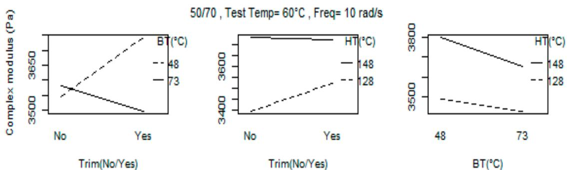
**Figure 1.** Two-level interaction plots for the  $G^*$  ( $\omega = 10 \text{ rad/s}$ ) at  $60^\circ\text{C}$  for 50/70.
