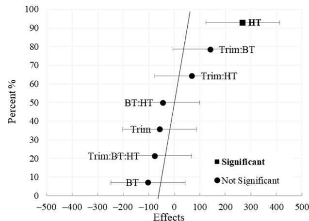
**Figure 2.** Normal probability of effect estimates at significance level of  $\alpha = 0.05$  for the  $G^*$  ( $\omega = 10$  rad/s) at 60 °C for 50/70.
