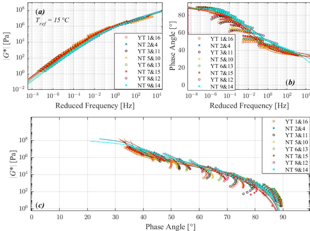
Figure 5. Comparison of master curves of complex shear modulus (a), phase angle (b), and black diagram (c) for 160/220\_I.
