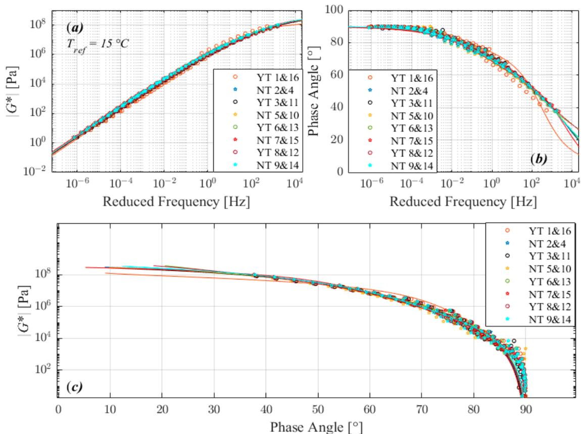
**Figure 6.** Comparison of master curves of complex shear modulus (a), phase angle (b), and black diagram (c) for 160/220\_II.
