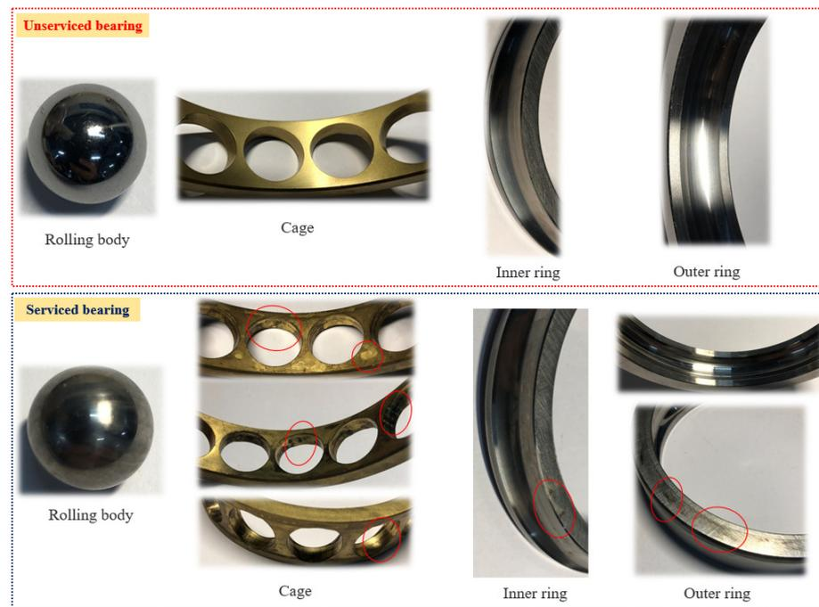
**Figure 6.** Naked-eye comparison of the surface conditions of high-performance bearings before and after the durability experiments.
