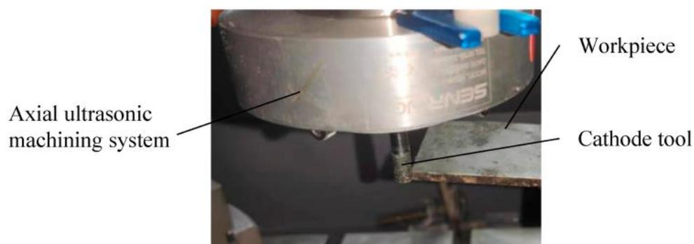
**Figure 4.** The machining area.
