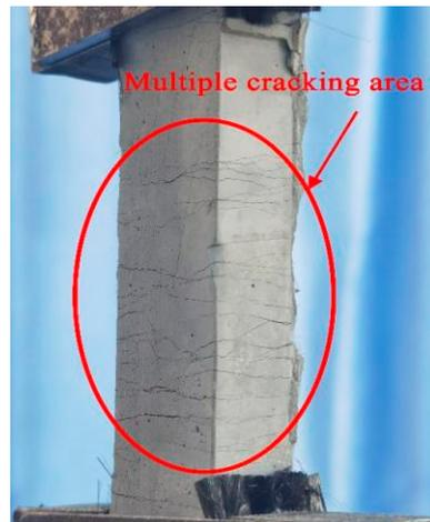
Figure 3. The cracking diagram of ECC.
