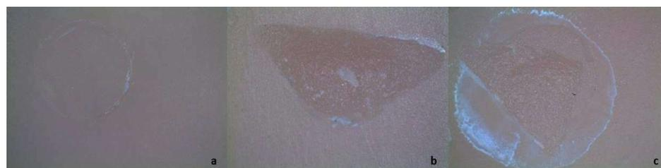
**Figure 2.** Stereomicroscopy photographs of the representative fracture patterns. Adhesive (a), cohesive (b), mix (c).
