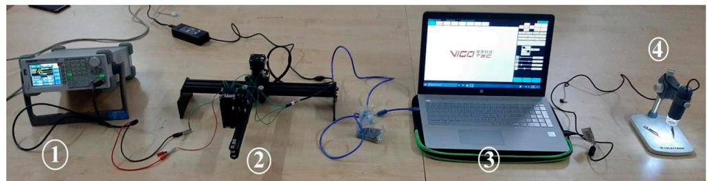
**Figure 2.** Machined buffalo leather samples under observation using a microscope: (1) waveform generator; (2) LBM setup; (3) software integration; (4) microscope.
