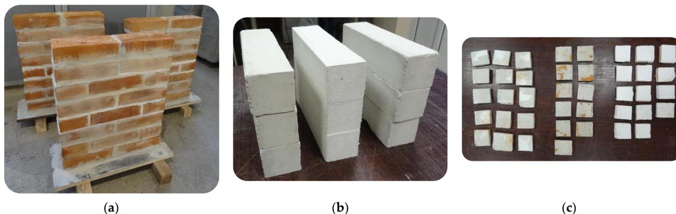
**Figure 4.** Tested elements: (a) brick masonry prisms; (b) standard specimens  $4 \times 4 \times 16 \text{ cm}^3$ ; (c) DPT specimens  $\approx 5 \times 5 \text{ cm}^2$ .
