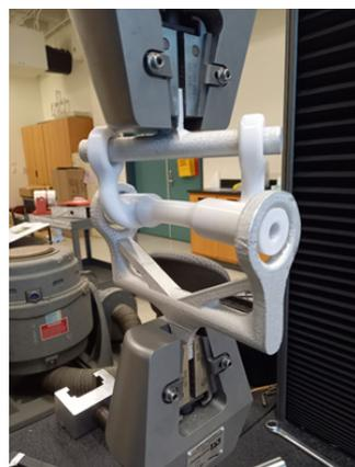
**Figure 19.** Combined loading specimen in the uniaxial test machine.
