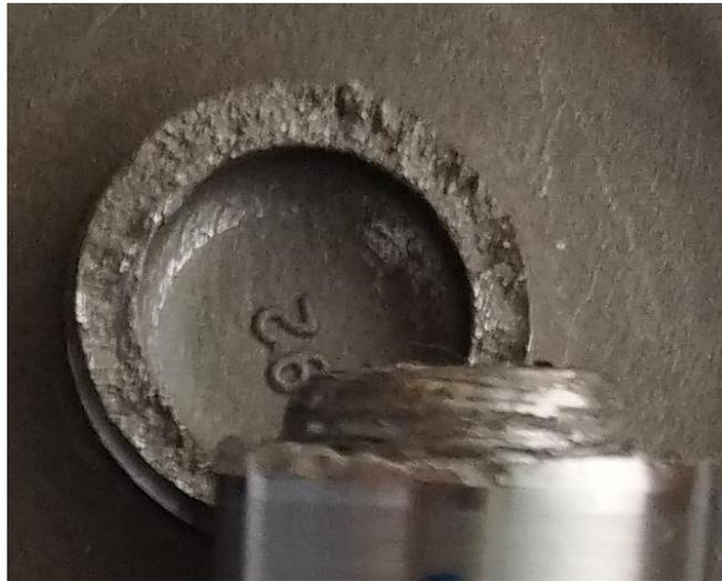
**Figure 12.** View of the sample fractured from the weld zone.
