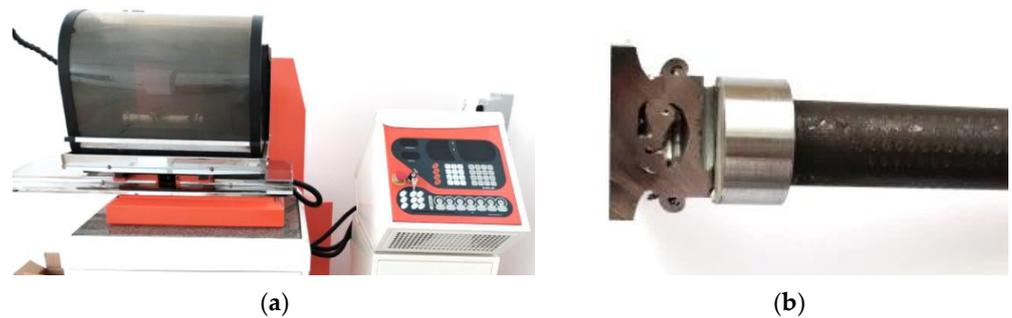
**Figure 8.** (a) BP95d electro-erosion cutter; (b) the place from which the samples were cut from the friction-welded rotor.
