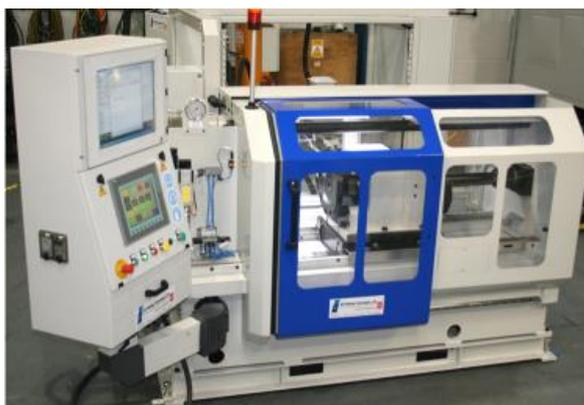
**Figure 4.** Friction welding machine MTI150B.
