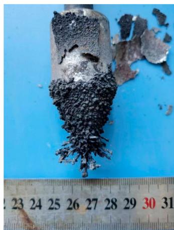
**Figure 8.** Zirconium cathode deposition products by electrolytic refining.
