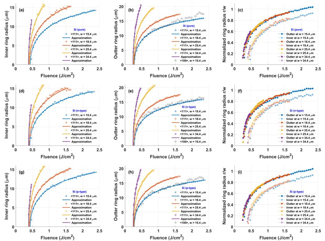
**Figure 3.** The inner (a,d,g), outer (b,e,h), and normalized (c,f,i) radii dependence on the fluence of laser pulse and beam focusing conditions. Circles depict the Si  $\langle 111 \rangle$  crystal orientation while squares depict the Si  $\langle 100 \rangle$  crystal orientation. The points correspond to the experimental measurements and the solid line to the approximation  $F_{thr}^{(i,o)} = F \exp(-r_{i,o}^2/w^2)$ . Silicon type: (a–c) no dopant, (d–f) n-type, (g–i) p-type.
