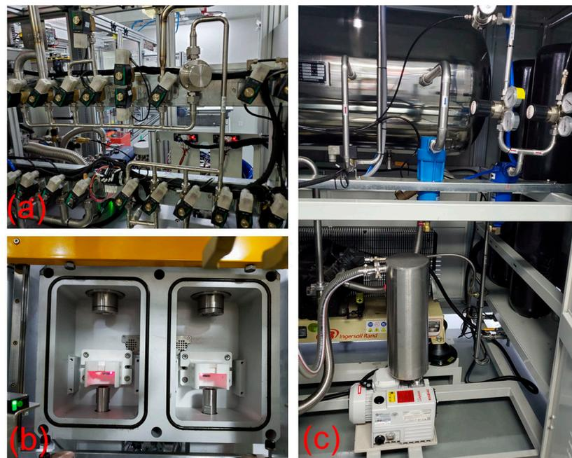
**Figure 4.** Helium leak test system: (a) Helium control valve; (b) vacuum test room; (c) helium recovery system.
