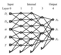
**Figure 2.** Schematic of ANN architecture. Nodes in each layer are indicated as square, circle, diamond, and triangle for the input layer, internal layers, output layer, and bias, respectively. Not all connections between adjacent layers are drawn.
