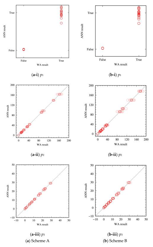
**Figure 4.** Comparison of predicted dislocation structures with the ANN and WA solutions for the training parameter sets of (a) Scheme A and (b) Scheme B. (i), (ii) and (iii) show Boolean values representing whether a dislocation wall structure is formed,  $p_1$ , the number of walls,  $p_2$ , and the average width of the formed walls,  $p_3$ , respectively. In (ii) and (iii), the red and faded red plots show the results after and before averaging with the same initial structure, respectively.
