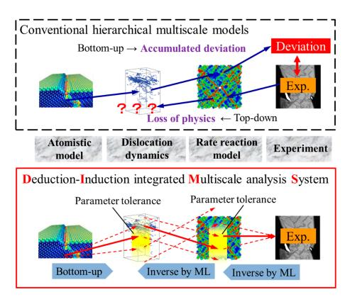
**Figure 6.** Schematic explaining the concept of suggested integration of deduction–induction approaches compared with conventional hierarchical multiscale models.
