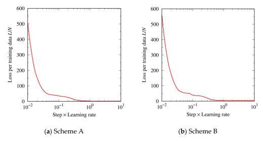
**Figure 3.** Loss function in (a) Scheme A and (b) Scheme B. The horizontal axis shows the value obtained by Step (max step is  $10^8$ ) × Learning rate ( $10^{-7}$ ). The vertical axis shows the loss per training data of the ANN model (N = 240).
