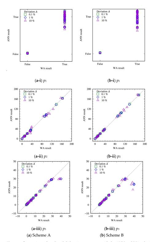
**Figure 5.** Comparison of predicted dislocation structures with the ANN and WA solutions for the deviated parameter sets of (**a**) Scheme A and (**b**) Scheme B. (i), (ii) and (iii) show Boolean values representing whether a dislocation wall structure is formed,  $p_1$ , the number of walls,  $p_2$ , and the average width of the formed walls,  $p_3$ , respectively. The square, diamond and triangle plots show the amount of deviation  $\Delta = 0.1$ , 1, and 10%, respectively.
