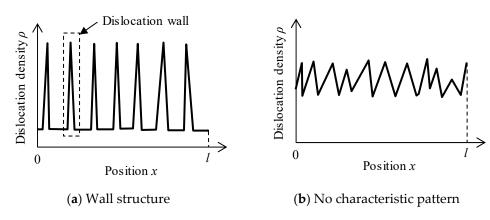
**Figure 1.** Schematics of typical dislocation density distributions ( $\rho_i$ ). (a): Aligned peaks with low-density areas in between, indicating formation of wall structure. (b): No self-organized dislocation pattern.
