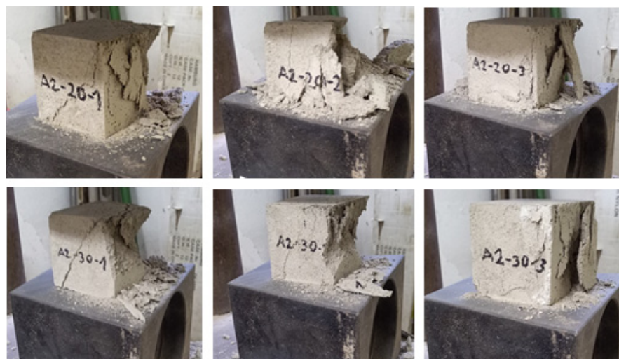
Figure 6. Impression of selected UCS specimens of the ash test series, here cubes having a filter ash share of 20 and 30%.
