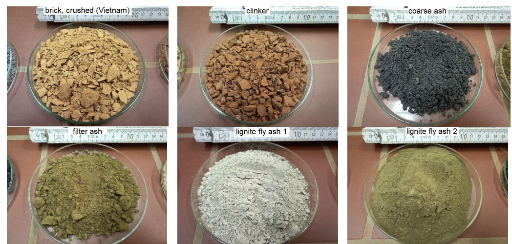
Figure 2. Potential secondary m-sand substitutes: crushed brick, crushed clinker; and secondary materials to substitute cement: lignite filter ash, coarse ash, and two types of fly ash (Figure source: Radek Kucera).
