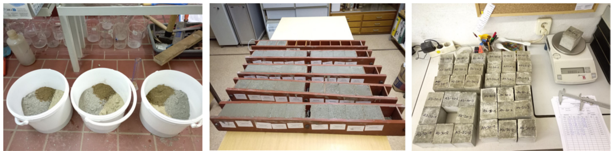
Figure 4. Manufacturing of the test specimens (Figure source: Radek Kucera).
