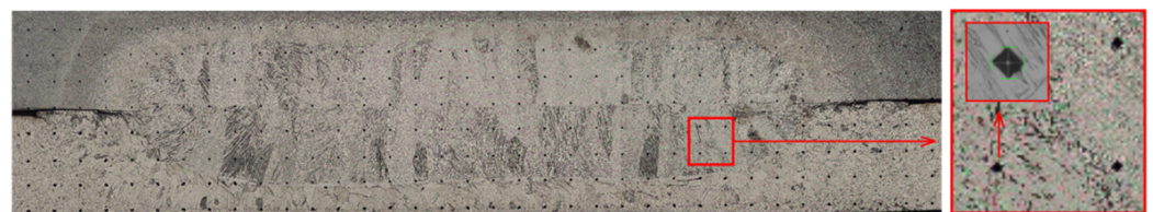
Figure 13. Maps of indentations after hardness measurement.
