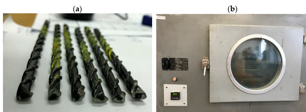
Figure 4. Preparation samples for mechanical tests; (a) One part of the samples prepared for the shear test, (b) The heating process of the samples at a stabilized temperature of 80° C.
