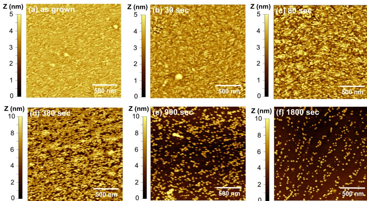
**Figure 5.** Atomic force microscope images exhibiting the progress of InGaN QD formation using PEC etching with a coherent light source at 0.4 V. The images are for the (a) as-grown surface and etched for (b) 30 s, (c) 80 s, (d) 380 s, (e) 900 s, and (f) 1800 s. The QDs formation is slower than at 0.9 V, and the QDs are fully formed at 380 s. QD density reduces from  $\sim 1 \times 10^{11}/\text{cm}^2$  at 380 s to  $\sim 1.2 \times 10^{10}/\text{cm}^2$  at 1800 s.
