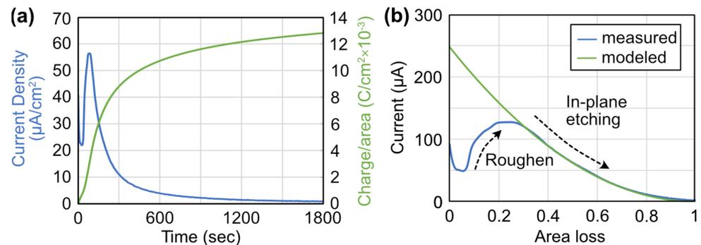
**Figure 8.** Plot of (a) current density and charge density versus time for an 8 nm thick InGaN layer at a potential of 0.4 V. The charge density is used to calculate the amount of InGaN volume etched over time. Plot of (b) measured and modeled current versus InGaN area loss at 0.4 V. At the initial stages of etching, the current increases due to surface roughening. The current can be modeled at higher area loss with a modified photoconductivity model.
