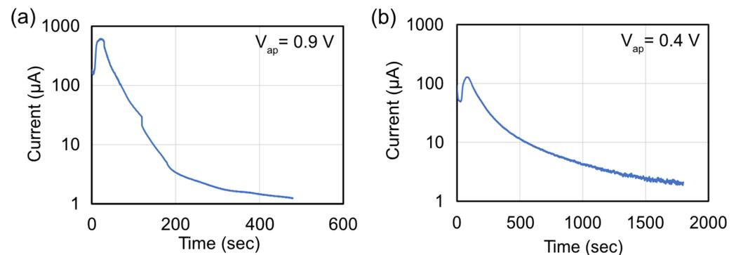
**Figure 3.** Etch current versus time at  $V_{ap}$  of (a) 0.9 V and (b) 0.4 V. (The discontinuities in (a) are caused by stopping the etch to measure AFMs.) At 0.9 V, the etch current has a higher peak and is completed in a shorter amount of time.
