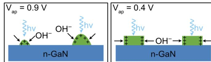
**Figure 1.** Cross-sectional schematics of the PEC etch process with a coherent light source with two different applied potential ( $V_{ap}$ ). The InGaN layer (green) absorbs the light, creating electrons and hole pairs, where the holes collect at the surface. Anisotropy in the distribution of holes creates anisotropic etching that depends on the applied potential.
