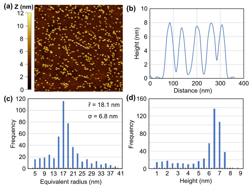
**Figure 6.** Atomic force microscope image (a) of QDs etched at 0.4 V for 30 min, similar to Figure 4f. A plot (b) of height versus distance for the cross-sectional line (white) in (a). Frequency versus bins of QD equivalent radius (c) and height (d) for the image shown in (a). The QDs have a tight distribution for radius with a mean value of 18.1 nm. The QD heights are concentrated at  $\sim 7.5$  nm, the initial InGaN thin film thickness.
