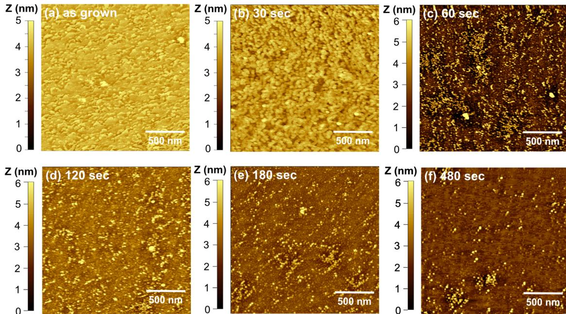
**Figure 4.** Atomic force microscope images showing the progress of InGaN QD formation using PEC etching with a coherent light source at 0.9 V. The images are for the (a) as-grown surface and etched for (b) 30 s, (c) 60 s, (d) 120 s, (e) 180 s, and (f) 480 s. The QDs form at 60 s and have heights that vary from 2 to 5 nm. As the etching time increases, the QD density decreases from  $\sim 7 \times 10^{10}/\text{cm}^2$  at 60 s to  $\sim 1.5 \times 10^{10}/\text{cm}^2$  at 480 s.
