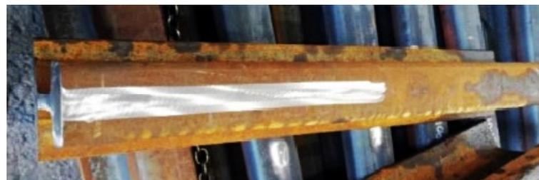
**Figure 14.** Rail head and foot prepared for welding. Source: own.
