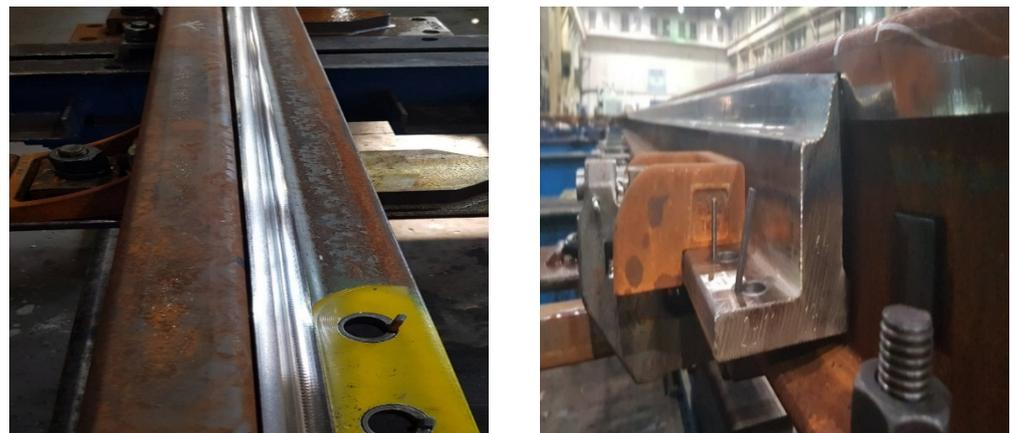
Figure 3. Adhesion of the needle to the stop. Source: own.
