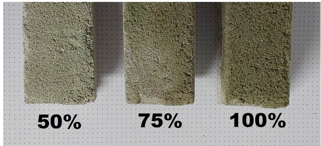
**Figure 4.** Examples of concrete samples with sewage sludge addition.
