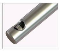
**Figure 2.** Close-up of the cutting principle of a vitrectome. The inner knife moves with a linear cutting motion within the stationary outer knife. Both knives have an opening on the side called an aspiration port, these two ports cause the inner knife to create two cuts instead of one per reciprocating motion (the cutting sides of the inner knife are highlighted with a blue line).
