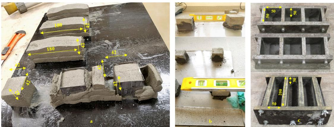
**Figure 3.** Sample preparation (a) for compressive and flexural strength measurement of printed members using the extruder, (b) preparing a flat surface for extruded samples for compressive strength test, and (c) moulds for preparing cast samples to test compressive and flexural strength.
