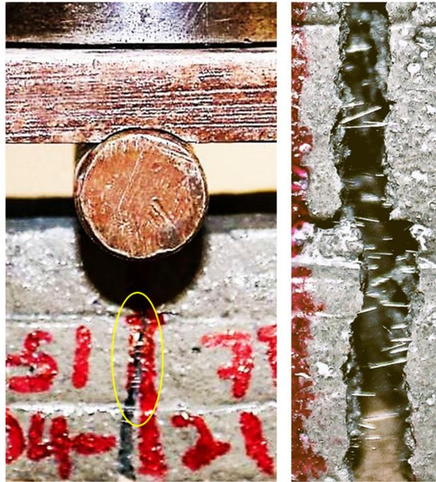
**Figure 13.** Basalt fibre aligned along the direction of printing and visible through the crack after failure in the 3-point bending test.
