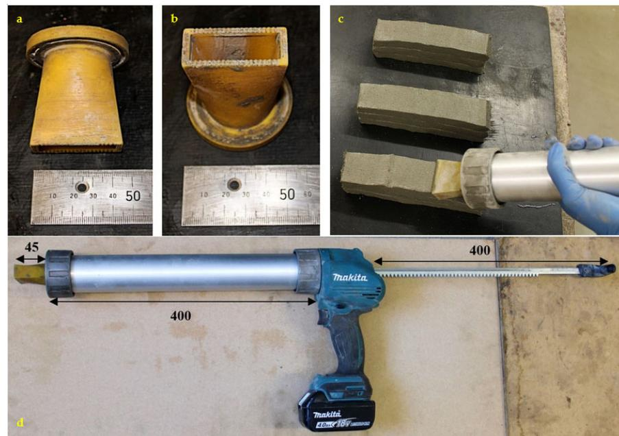
**Figure 2.** The printing system used for printing of mortar (all dimensions are in mm): (a) side view of the nozzle, (b) front view of nozzle, (c) battery operated ram extruder device fitted with nozzle, and (d) a few printed sample later used for flexural strength test of extruded samples.
