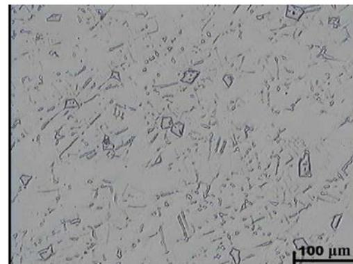
**Figure 8.** As-cast microstructure obtained in the alloy with 9.2% Nb addition; austenitic matrix with primary niobium carbides; etched with Mi16Fe.
