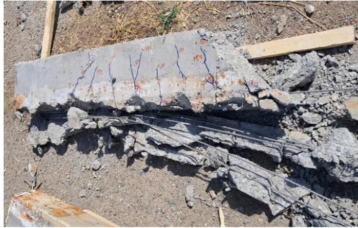
**Figure 7.** Destruction of specimens and removal of prestressing wires.
