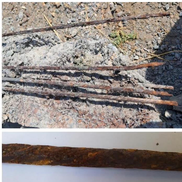
**Figure 6.** Corroded prestressing wires.
