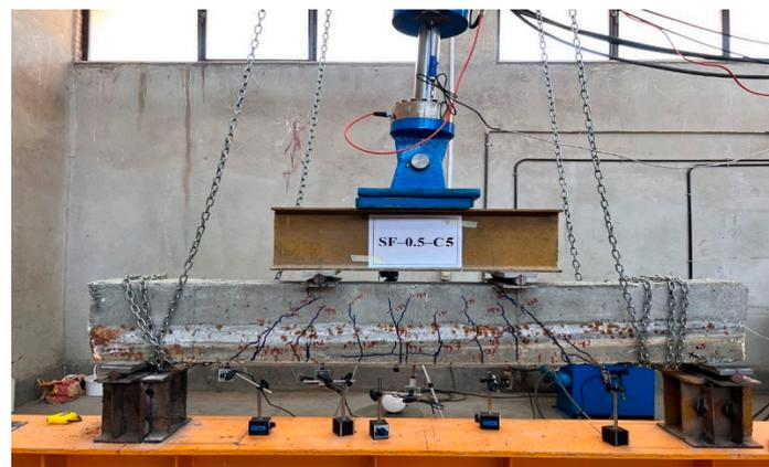
Figure 8. Four-point bending test setup.
