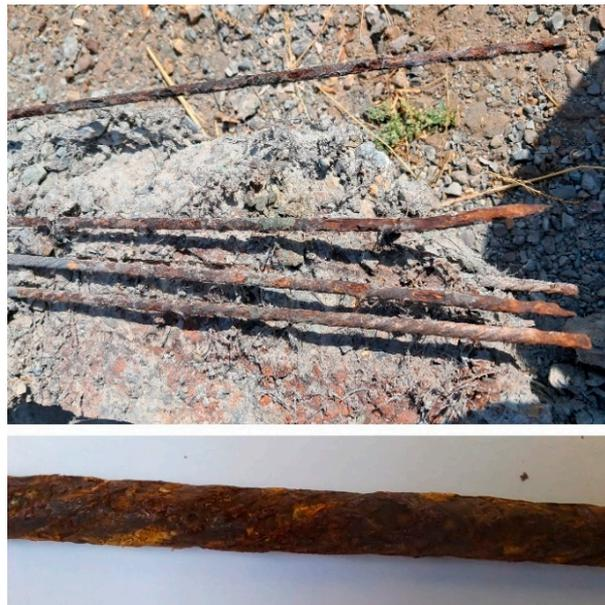
Figure 6. Corroded prestressing wires.
