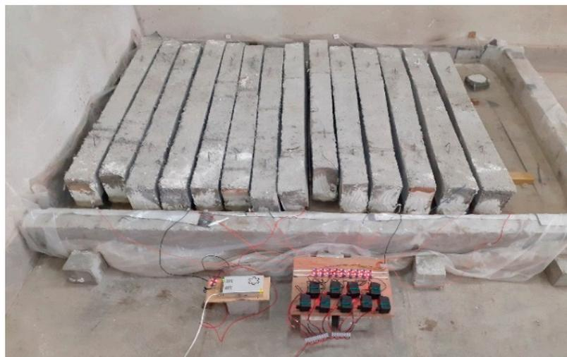
**Figure 4.** Accelerated corrosion of the prestressed concrete beams.
