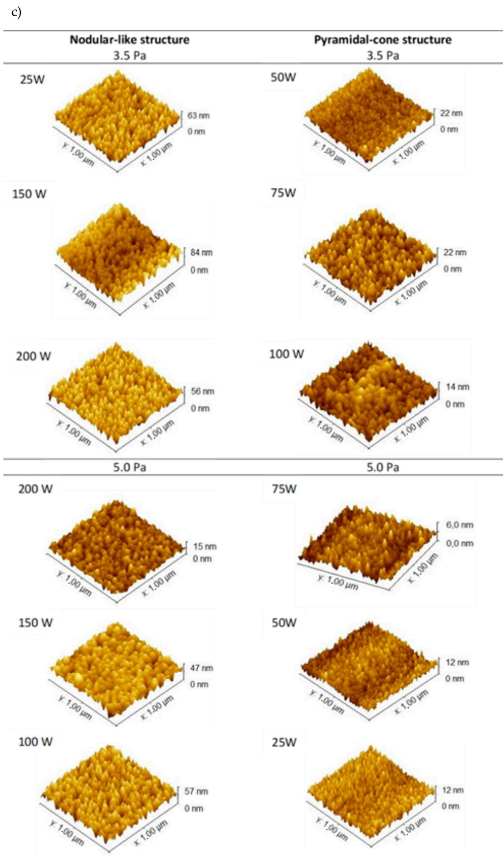
**Figure 5.**  $1 \times 1 \mu\text{m}^2$  2D AFM micrographs of the sputtered  $\text{Cu}_3\text{N}$  films deposited at different RF powers and at (a) 3.5 Pa and (b) 5.0 Pa; (c)  $1 \times 1 \mu\text{m}^2$  3D AFM micrographs divided depending on the type of morphology.
