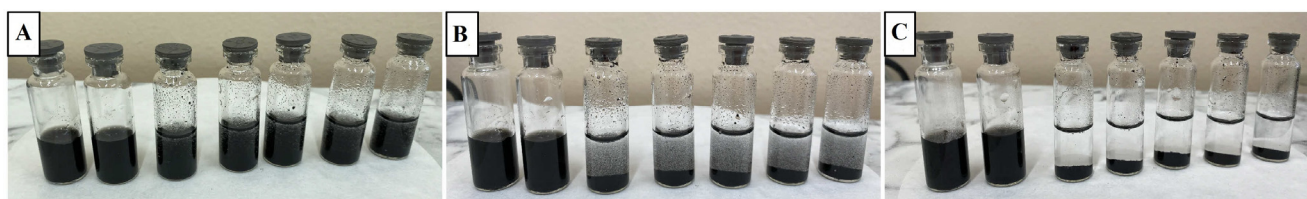
Figure 1. Stability of aqueous suspensions of MWCNTs. (A) Immediately after dispersing in an ultrasonic bath, (B) after 1 h exposure, (C) after a week. From left to right: MWCNT-1-ox (0.6), MWCNT-2-ox (0.5), MWCNT-1, MWCNT-1 (0.6), MWCNT-2, MWCNT-2 (0.5), and MWCNT-3.
