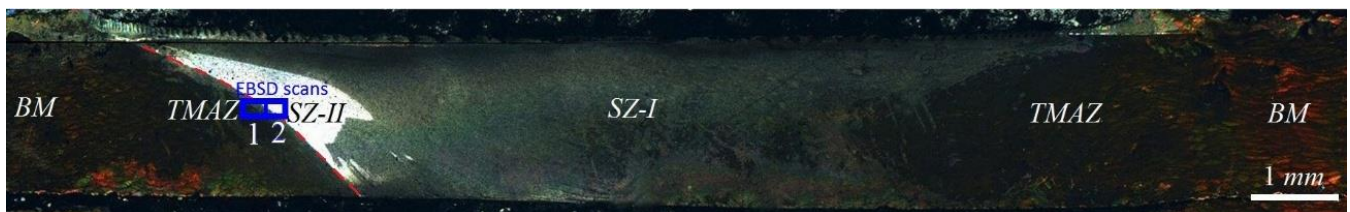
Figure 7. Cross-sectional macrostructure of 2-pass friction stir processed sample. The blue rectangles indicate areas 1 and 2 of EBSD scans. The details of the FSP reference frame are the same as Figure 2. The interface between TMAZ and SZ is depicted by a red-dashed line.
