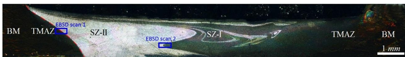
Figure 10. Cross-sectional macrostructure of 3-pass friction stir processed sample. The blue rectangles indicate the areas of EBSD scans. The details of the FSP reference frame are the same as Figure 2. Interface between TMAZ and SZ is depicted by a red-dashed line.
