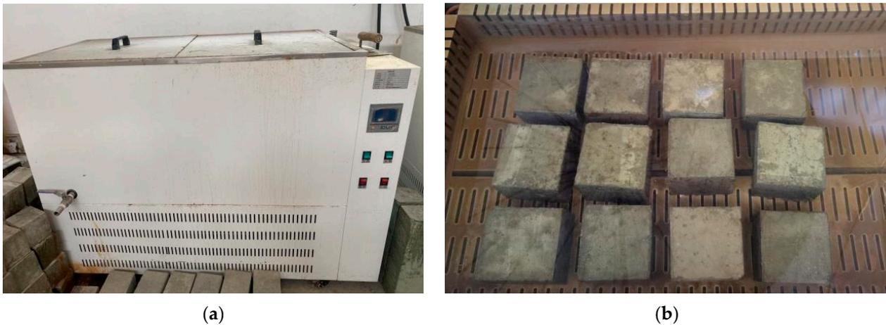
**Figure 2.** Drying–wetting cycle: (a) apparatus for soaking specimens; (b) part of specimens immersed in the chloride solution.
