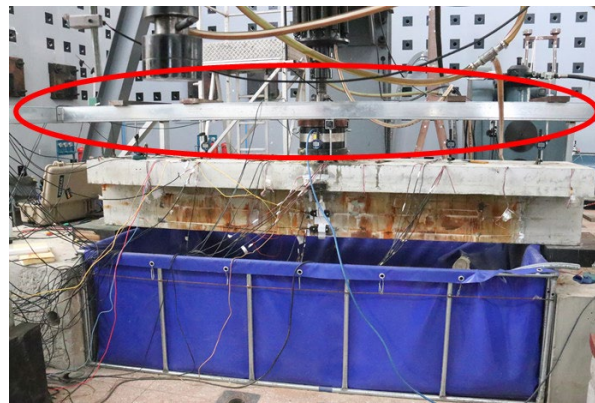
Figure 8. Square steel frame.
