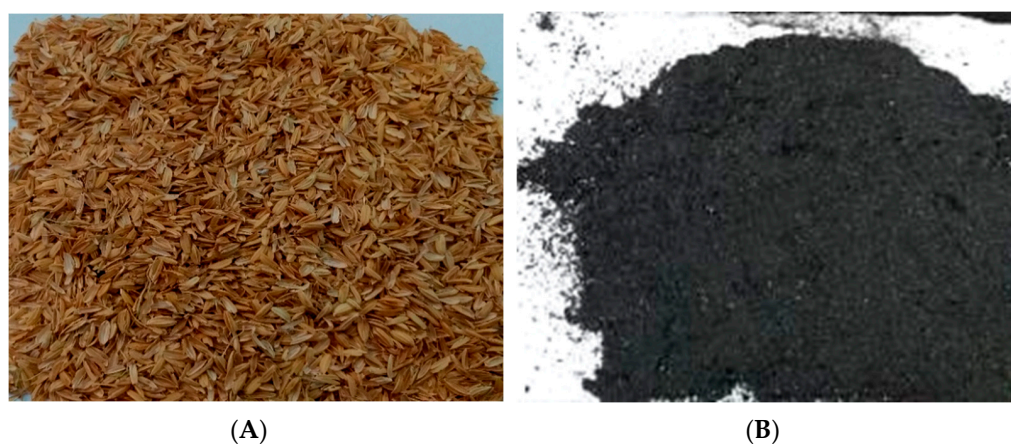
Figure 1. Photographic pictures for (A) raw rice husk (RH) at 25 °C, (B) rice husk (RH) AC carbonized at 700 °C (AC(C-3)).
