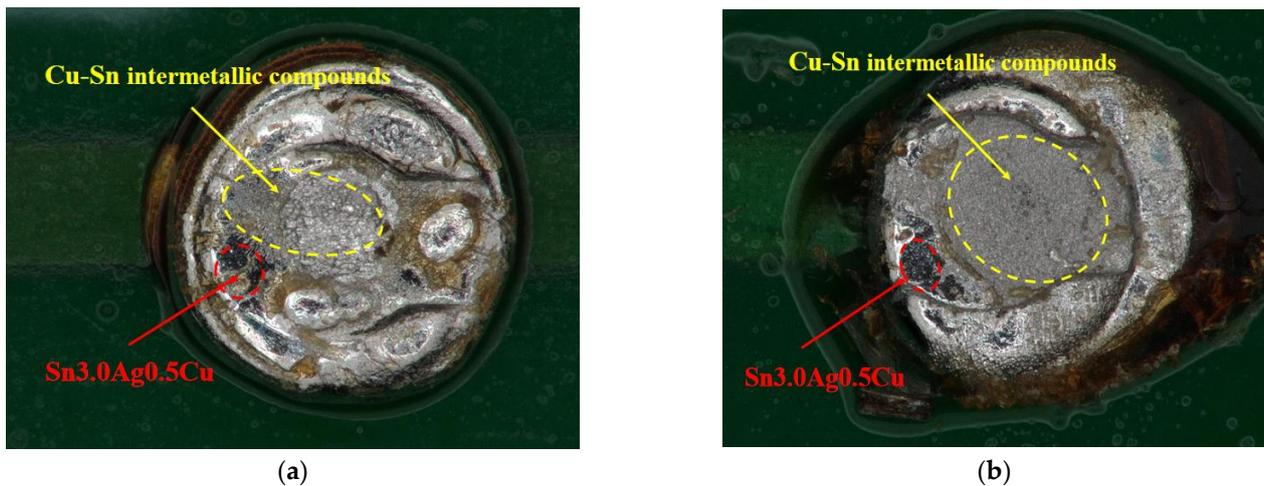
**Figure 7.** Fracture surfaces of Cu/Sn3.0Ag0.5Cu/Cu. (a) The cathode side. (b) The anode side.
