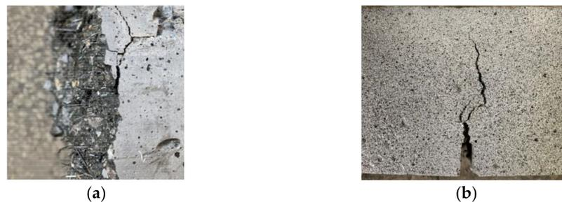
**Figure 7.** Steel fiber distribution in cross section and crack development of notch. (a) Steel fiber distribution in the cross section; (b) Crack development of notch.
