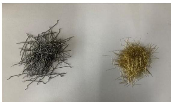
**Figure 1.** End-hooked steel fiber (left) and straight steel fiber (right).
