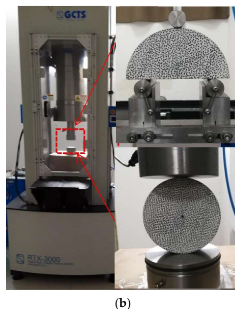
Figure 1. Configuration of rock specimens and testing machine. (a) Top: notched semi-circular bending (NSCB) specimens; (b) bottom: center-cracked circular disk (CCCD) specimens.
