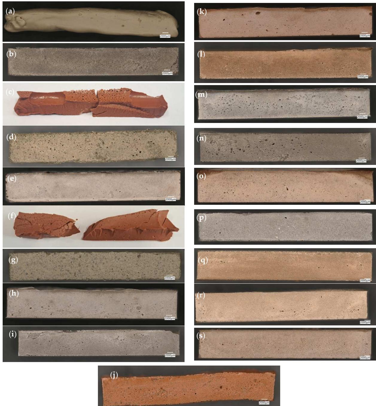
**Figure 1.** Obtained geopolymer binders based on waste materials: (a) R.Ch; (b), R.PB; (c) R.D; (d) R.A; (e) R.M; (f) Ch + D; (g) Ch + A; (h) Ch + M; (i) Ch + PB; (j) D + A; (k) D + M; (l) D + PB; (m) A + M; (n) A + PB; (o) Ch + D+A + M; (p) Ch + A + M + PB; (q) Ch + D + A + PB; (r) D + A + M + PB (s) Ch + D + M + PB.
