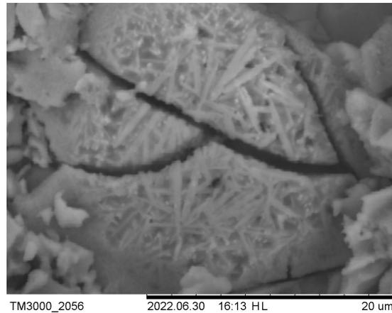
**Figure 16.** At a temperature of 1200 °C, sintered CS1-0 cenospheres (CP 250 bar).
